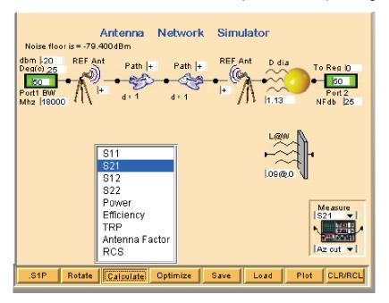
The 1.1m sphere is the standard for dBsm and has a frequency independent reflection crossection of  $1m^2$
