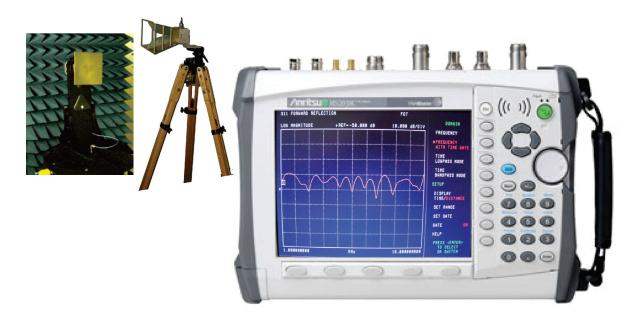
With the DAMs Azimuth set to 0-360 with 10 degree steps, load the RCS measurement schematic and invoke the FSM RCS measurement/calculation. Minus (-) is de-embed.
