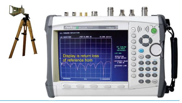
Initiate time domain and distance. Notice the S11 drops to below -50dB at distance compared to the -10dB at near 0m(the horn reflection). With the plate reference at right angle (Use DAMs jog) store the trace into memory and display data and memory. The rotate the plate to full reflection and observer the position with the marker(1.25m) set to the peak change.
