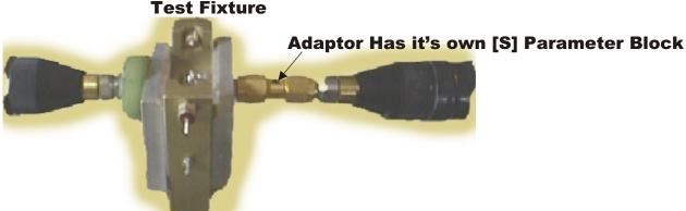
The adaptor S-Parameters are measured using a Teflon SMA barrel whose length is known. This allows the S-Parameters of the two piece assembly to be measured. The Adaptor [S] matrix is extracted by subtracting the delay of the barrel based on length. The coaxial loss is reduced by the same ratio. This assumption relies on near perfect impedance and match. Both sections must have the same basic physical structure.
