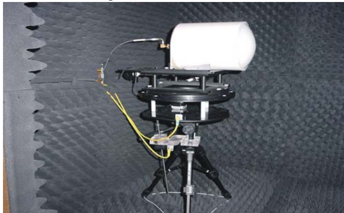
Fig 1-10 Anechoic antenna measurement chamber constructed for very high microwave frequency antenna measurements (Courtesy of Motorola)
