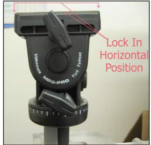
2. Place the tripod head in a horizontal position and tighten the locking screw.
