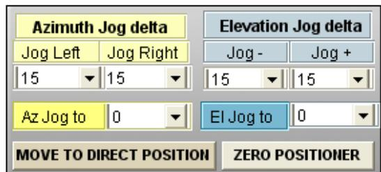
The screenshot shows a software interface with several controls for the positioner. It includes two columns of jog delta settings: Azimuth Jog delta (Jog Left and Jog Right) and Elevation Jog delta (Jog - and Jog +). Below these are two pull-down menus for 'Az Jog to' and 'El Jog to', both currently set to 0. At the bottom, there are two buttons: 'MOVE TO DIRECT POSITION' and 'ZERO POSITIONER'.
