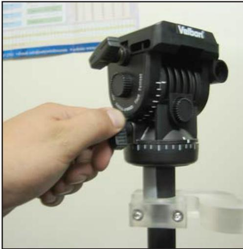
1. Ensure the azimuth setting on the tripod is unlocked.
