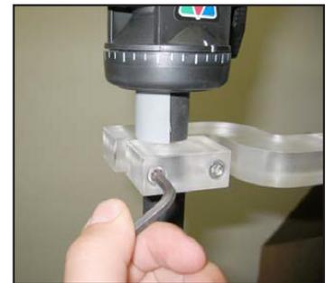
Attach vertical assembly ensuring vertical actuator rod does not hit tripod legs as it moves down
